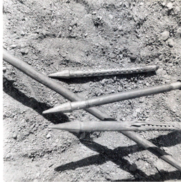
Top well-point, slightly bent, is heavy duty type. Bottom well-point is brass-jacket type with ripped screen.
